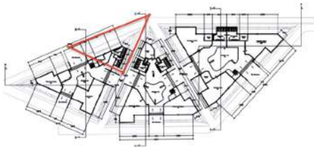
Fig. 1. RF Project with the triangular corners of the building floor plan was cut to fit the standard rectangular shape of the public toilets floor plan. Source: Department of Architecture, Hasanuddin University [38].
